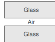
Fig. 15.3 Thin film of air formed between two glass plates.
