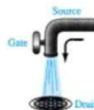
Figure 5.3 Water analogy for the JFET control mechanism.
